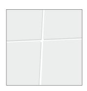
8. The grouting material should be applied 24/48 hours after the covering application, in order to help the evaporation of the water used to prepare the bonding mixture. This way is possible to avoid moisture stains that might end up causing efflorescence pathologies.
